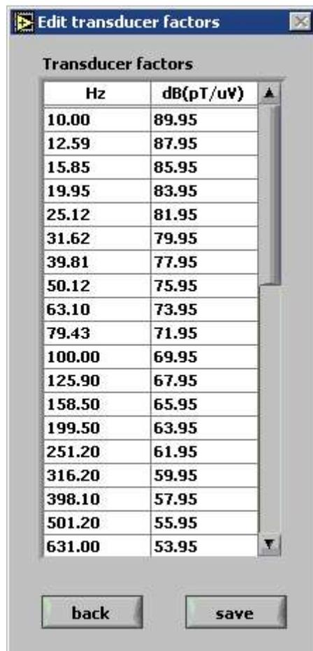
*Sensor loop calibration file is editable in this window*
