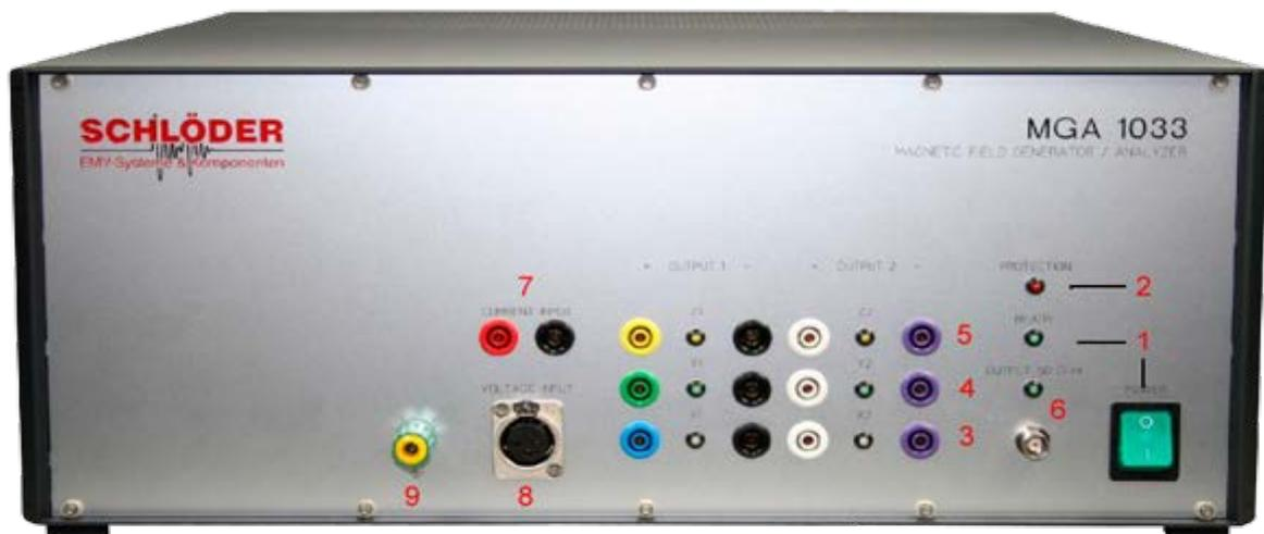
**[1]: POWER switch** Turns the MGA 1033 on and off.
