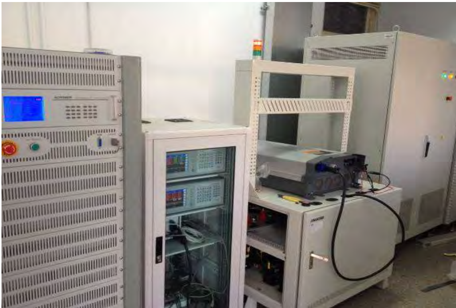
50kW PV Inverter Test System
