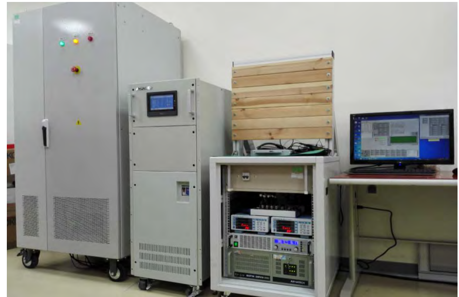
5kW Micro Inverter Test System
