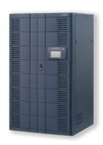
Adopting digital control technology, the ABU series on-line industrial UPS will continuously monitor working status and battery condition, and alarm if failure occurs. ABU can filter mains input noise and provide pure sine wave power to loads. The output isolation transformer can further improve overload capability and help ABU to sustain impact current.
