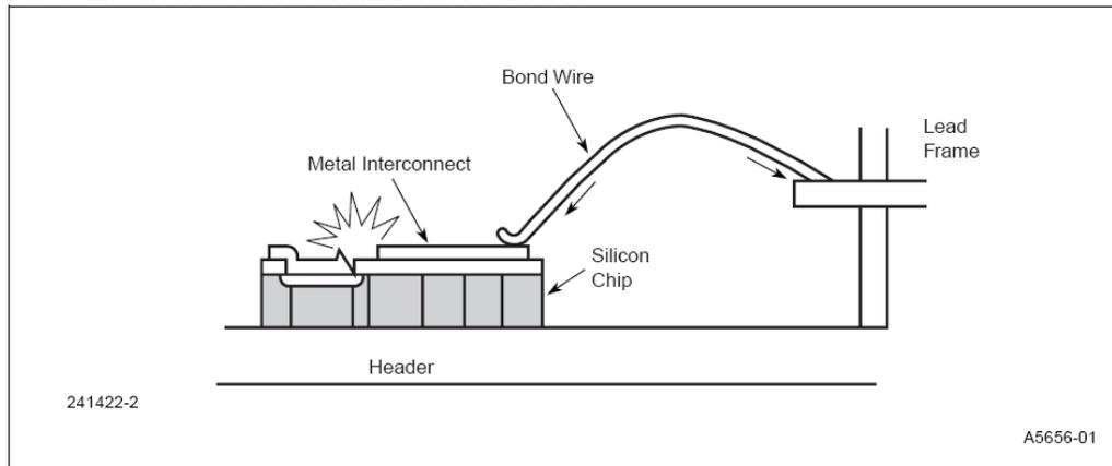
**Figure 3-3. Open Bond Wire Failure**
