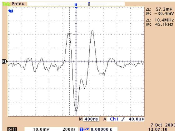
Figure 5. Current in GBB (gold ball bonding) Tool (peak current is 182mA)
