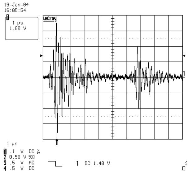
Figure 3. Voltage between the tip of a tool and ground.
