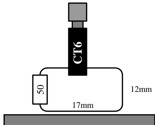
Figure 8. Configuration of Test Loop
