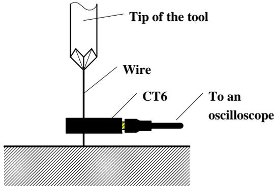
Figure 4. Current Measurement Setup in the Tool
