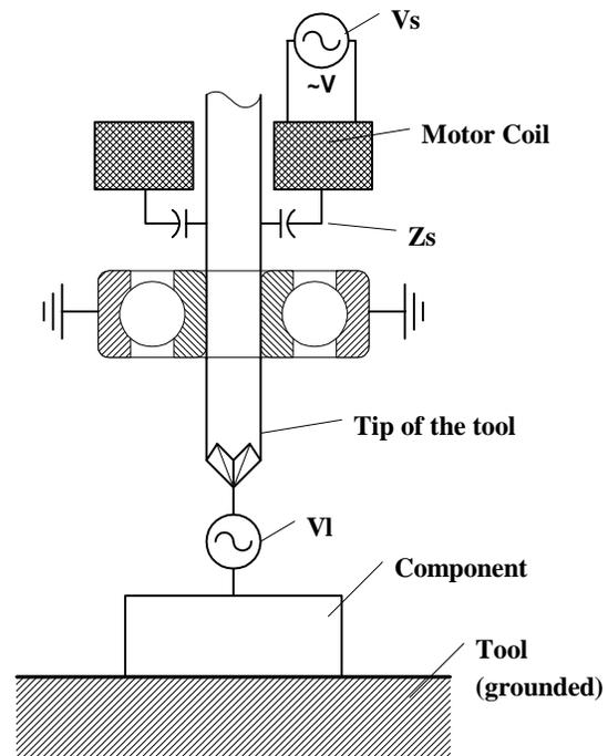
Figure 2. Generation of Voltage in a Tool via Capacitive
