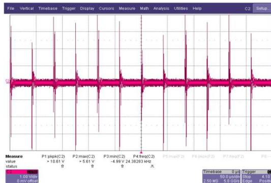
Figure 9a. Ground Current in Servo Motor without Filter: 1.12A
