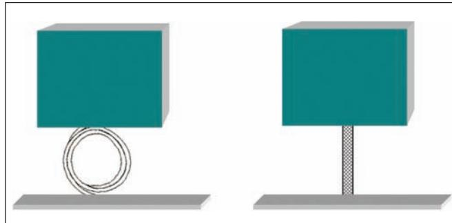
**Figure 3: Grounding with High and Low Impedance Path**
