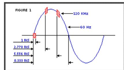
Figure 3. Example of PLC: X10
