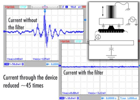
Figure 14. Reduction of EOS current using SF-series filter
