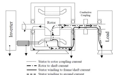
Figure 4. Parasitic current path in a motor
