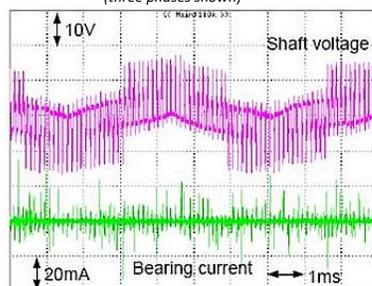
Figure 5. Shaft voltage and bearing current
