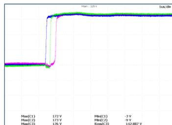
Figure 3. Pulse edges of servo drive signal (three phases shown)
