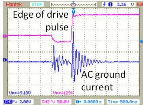
Figure 7. AC ground current caused by operation of a servo motor
