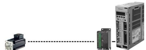
Figure 12. Place filter close to the controller, not to the motor
