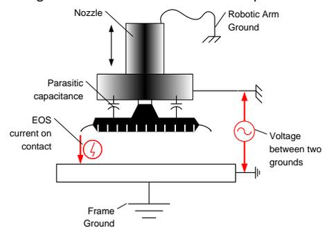
Figure 9. Unwanted current through IC in a handler
