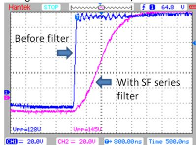
Figure 12. Typical edge modification of servo drive signal by a SF series filter
