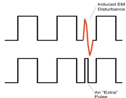
Figure 8. Illustration of how EMI corrupts data
