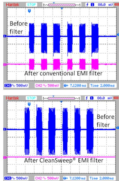
Figure 10. Power line communication signal with conventional filter (top chart) and with OnFILTER's CleanSweep® EMI filter (bottom chart)
