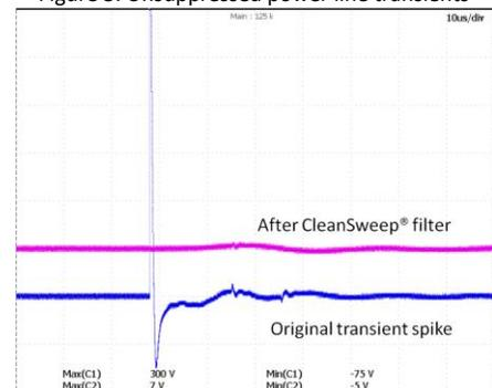
Figure 4. CleanSweep filter suppression performance
