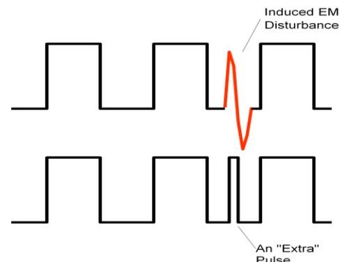
Figure 8. Mechanism of data corruption by EMI
