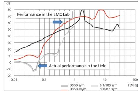
Figure 11. Frequency response of a conventional EMI filter
