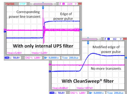
Figure 7. CleanSweep filter reduces EMI from UPS on AC mains
