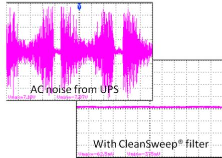
Figure 9. CleanSweep® filter reduces output transients from UPS
