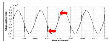
Figure 3. Unsuppressed power line transients
