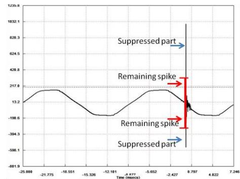
Figure 2. "Suppressed" power line transient
