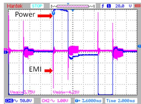
Figure 5. Power line transients from UPS
