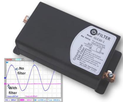
Figure 1. GLE30-1 Ground Line EMI Filter
