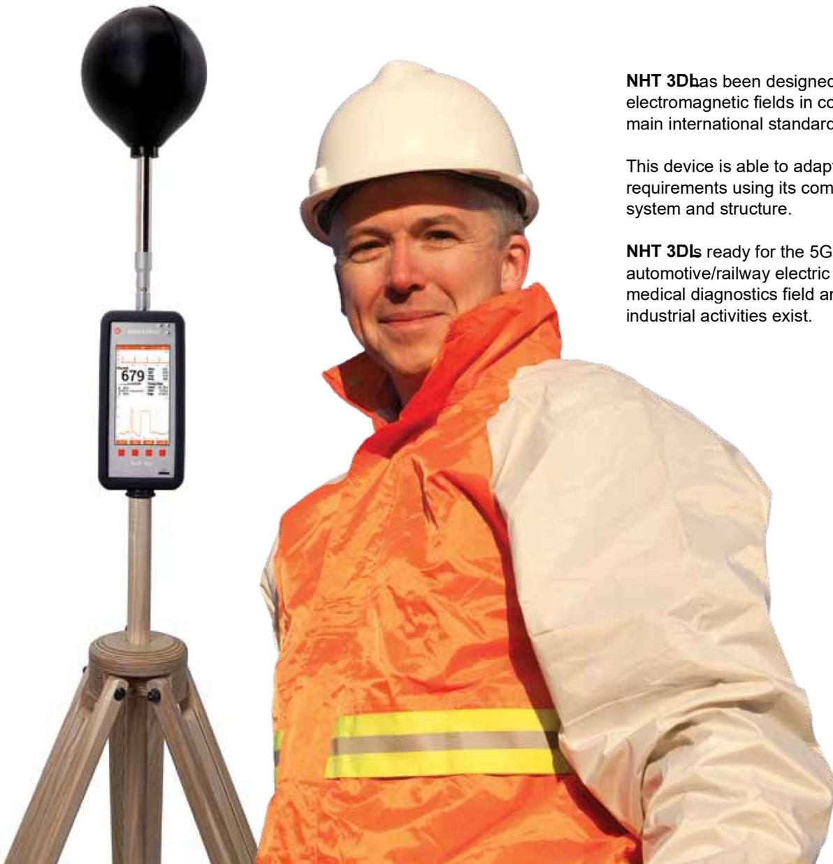
**NHT 3Di** has been designed to measure electromagnetic fields in compliance with all the main international standards and regulations.
