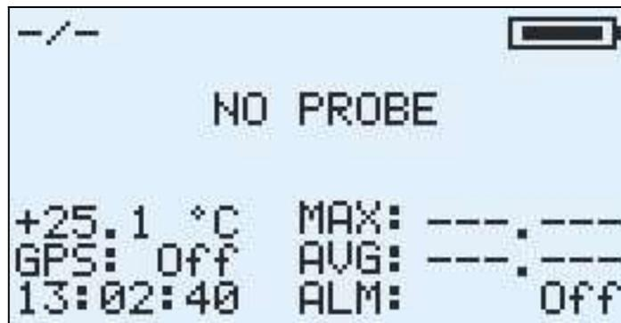
Fig. 6.5 – Typical screen in case of probe absence
