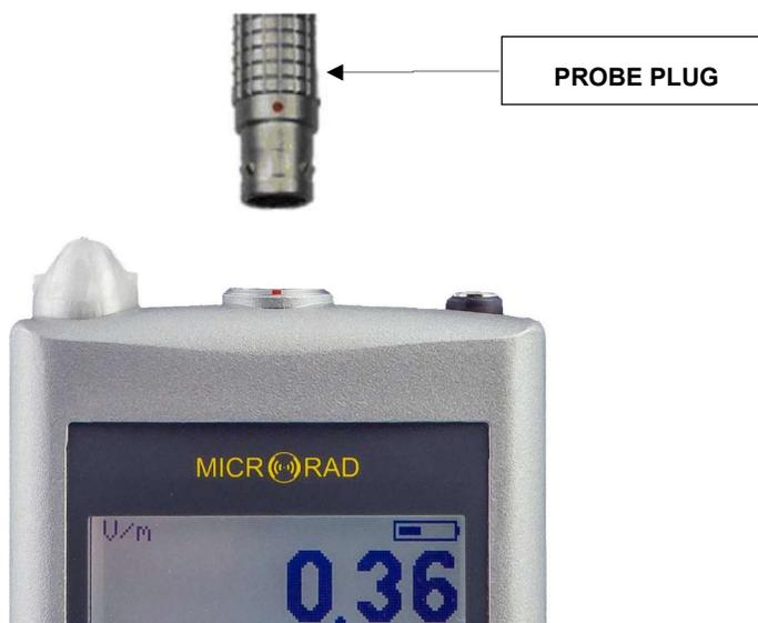
Fig. 5.1 – Probe connection
