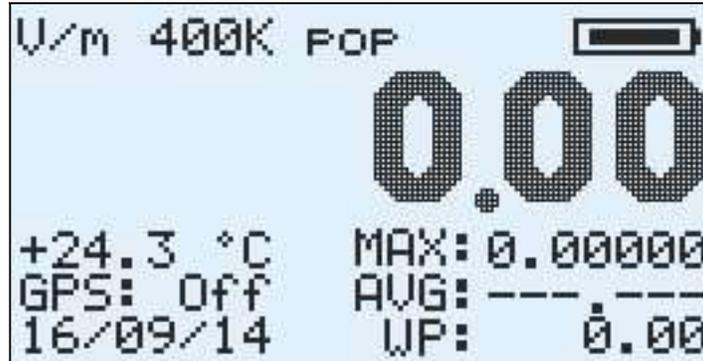
Fig. 6.4 – Typical screen during calibration
