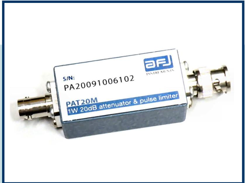
This 20dB attenuator is designed for pulse voltages up to 1Ws, to protect the input receivers. Even using EMI Test systems already protected against spikes, for unknown devices under test, the PAT 20M pulse limiter is strongly recommended.
