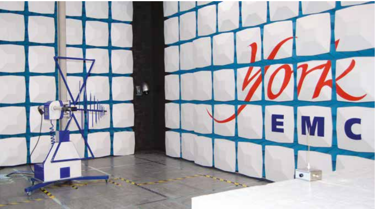
Figure 2. Radiated emissions pre-test check in operation
