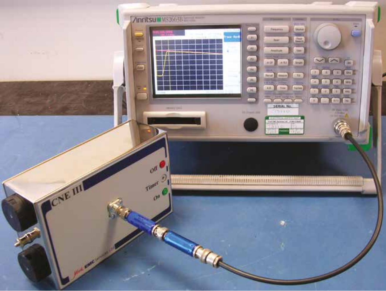
Figure 1. Measurement of 100 MHz high-pass filter using a CNE III
