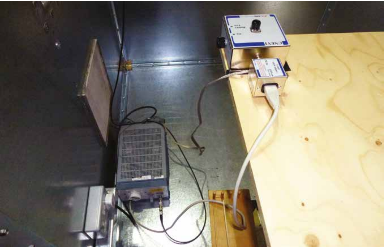
Figure 3. LISN verification setup using a CNE
