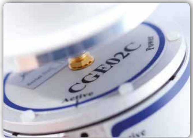
Comb Generator Emitters (CGEs) Reference Signal Source
