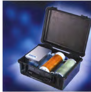
Figure 17. DIEHL Munitions damped sine IEMI generator
