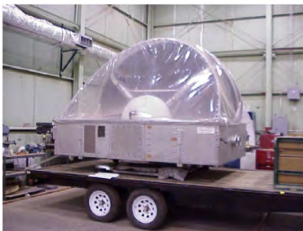
Figure 20. High intensity JOLT hyperband generator used in the United States
