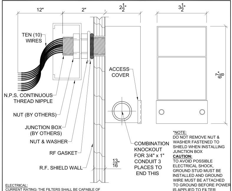
CURRENT RATING: THE FILTERS SHALL BE CAPABLE OF WITHSTANDING 140 % OF RATED CURRENT FOR 15 MINUTES WITHOUT ANY DETERIORATION.
