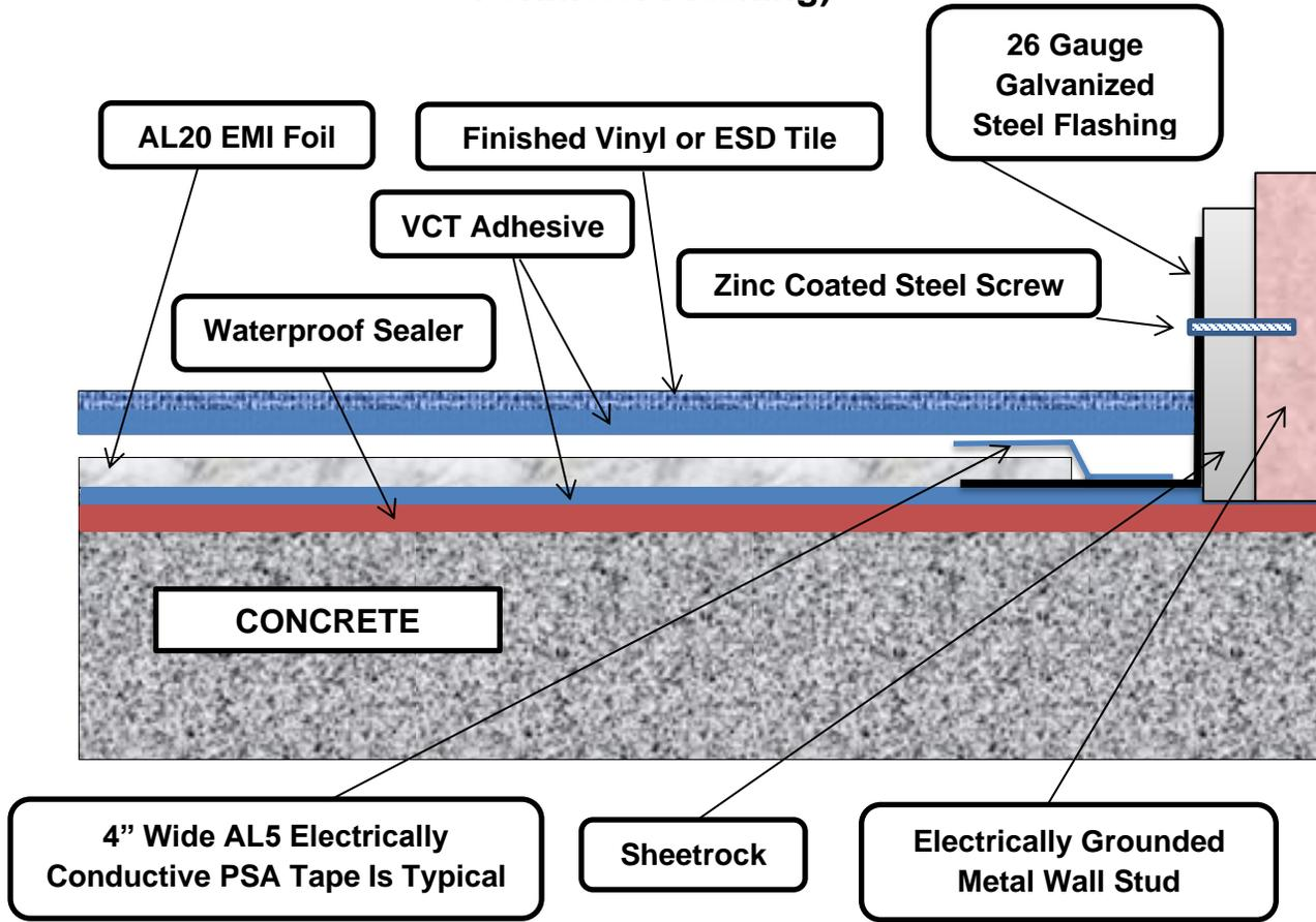
4" x 4" or 6" x 6" 26 Gauge Galvanized Steel L Flashing is Typical
