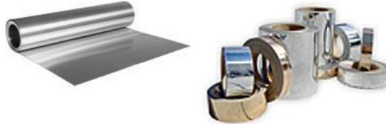
**EMI-SHIELD AL2.5** is a 0.0025" (2.5 mil) (0.0635mm) thick aluminum foil for use as an EMI/RFI shield against electromagnetic interference. The foils are easy to work with and offer good shielding effectiveness across a wide range of frequencies, shielding against unwanted signals in or out of rooms and buildings.
