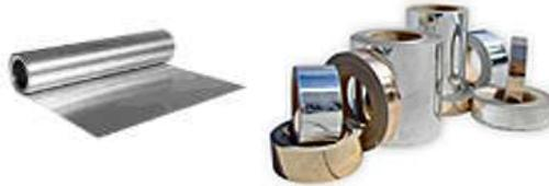
**AL5** is a 0.005" (5 mil) (0.127mm) thick aluminum foil for use as an EMI/RFI shield against electromagnetic interference. The foils are easy to work with and offer good shielding effectiveness across a wide range of frequencies, tested from 9 KHz to 40 GHz, shielding against unwanted signals in or out of rooms and buildings. Ideal for ICD 705 Tempest shielding.
