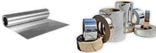
**EMI-SHIELD AL5** is a 0.005" (5 mil) (0.127mm) thick aluminum foil for use as an EMI/RFI shield against electromagnetic interference. The foils are easy to work with and offer good shielding effectiveness across a wide range of frequencies, tested from 9 KHz to 40 GHz, shielding against unwanted signals in or out of rooms and buildings. Ideal for ICD 705 Tempest shielding.
