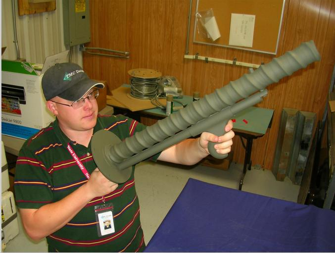
The HE-238-165-HH is a hand held directional antenna. The antenna is constructed entirely of aircraft certified 6061-T6 aluminum and G-10 fiberglass with copper radiator in a 100% sealed radome. This antenna was custom matched from 1.2 to 1.6 GHz to have the lowest VSWR possible, achieving a 2:1 VSWR across the band. The antenna is designed to provide many years of service.
