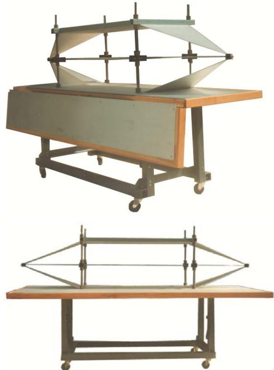
**The TDK TP-02 Triplate and integrated table is specifically designed to generate fields for EMC testing in automotive component test environments.**
