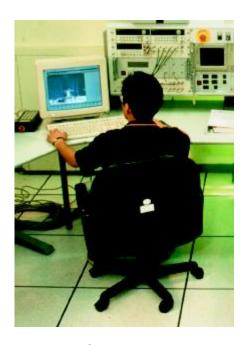
A TDK RF Solutions EUT Monitoring System integrates monitoring instrumentation, video and audio equipment, and software to provide EUT signal monitoring, EUT stimulation, and monitoring for visual or audio interference during testing.
