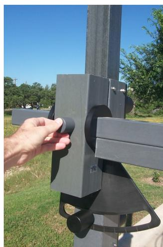
5. Replace polarization locking pin.
