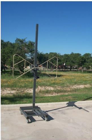
1. Antenna mounted on mast in horizontal polarization.
