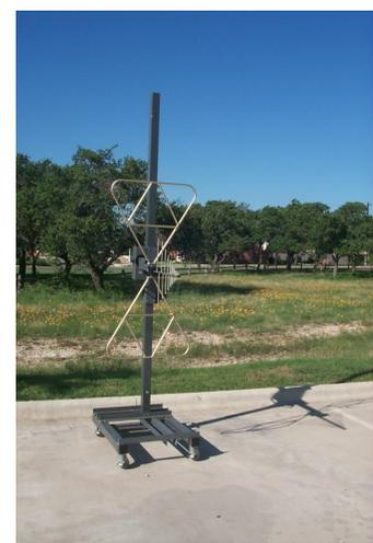
6. Antenna mounted on mast in vertical polarization.
