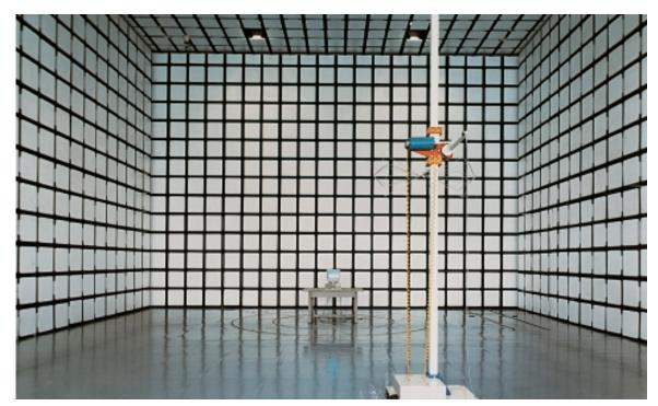
10 meter test range semianechoic chamber constructed by TDK utilizing IP-130BL absorbers.
