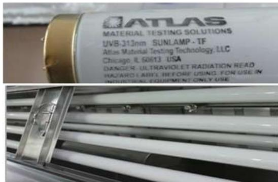
The UV lamp using ATLAS, spectral power distribution (SPD) will not change with the lamp aging and longer life
