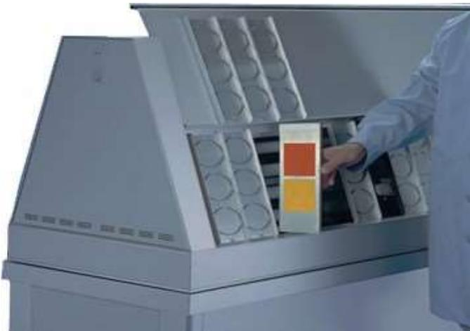
QUV tester can easily accommodate up to 48 samples (75mm x 150mm), fully in line with international, national and industry standards, to ensure that the test program reliability and reproducibility
