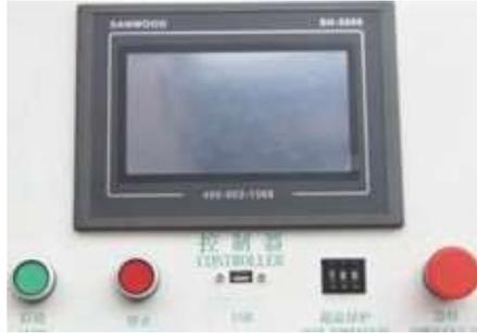
1. SH-5600 Controller , multi-function on control panel , battery surface temperature detection indicators , Battery fault alarm , Hazardous gases exceeding warning.
