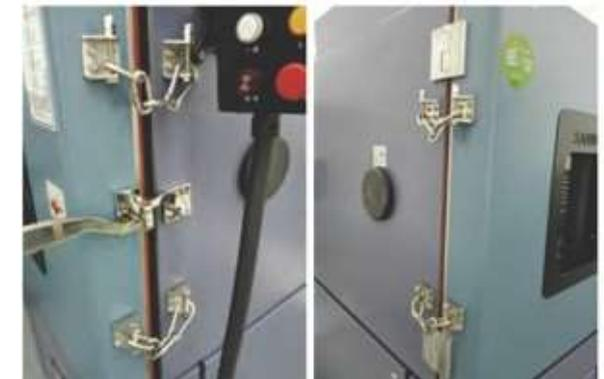
Using Explosion-proof lock and 2 Explosion-proof chains on each side for double protection.
