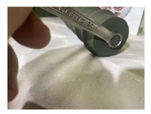
Remove for unpressurized operation, using a ½" wrench. When replacing DO NOT OVERTIGHTEN
