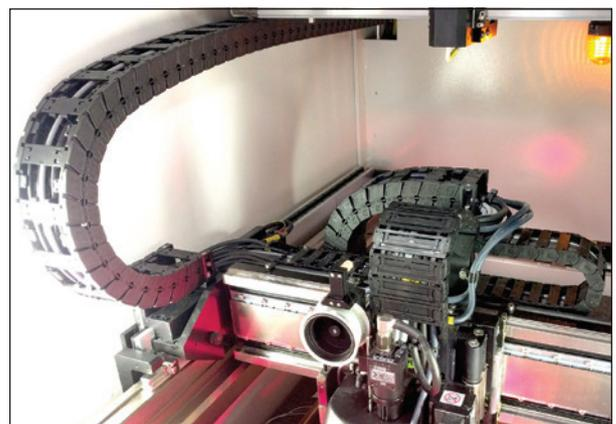
Figure 3: Flex cables on a robotic arm
