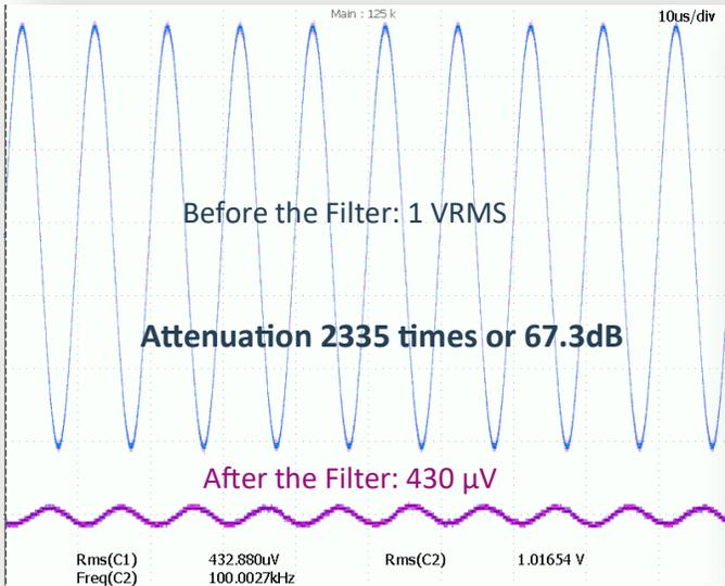
Typical DM Attenuation at 100 kHz (SPMS Range)
