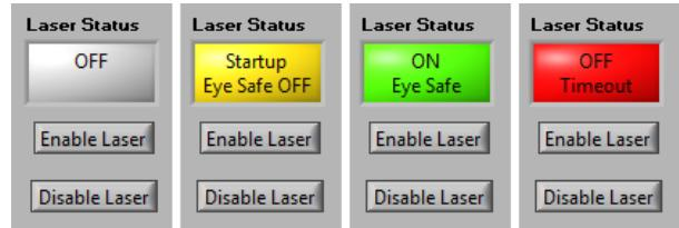
The GUI indicates proper operation by displaying a green "Laser Status" indicator as shown above. Stable operation is indicated by the Computer Interface's continuously on "Power", "Laser on" and "Data Link" LEDs as shown below.
