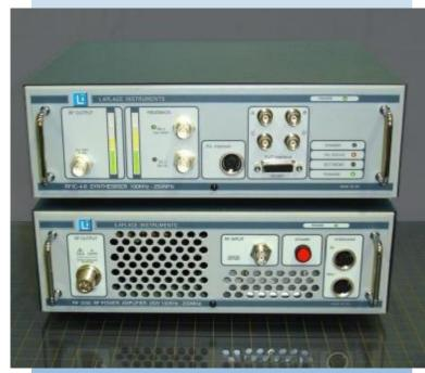
**Comprehensive** The system includes signal generator, power amplifier, RF detector/ millivoltmeter, USB interface, PC software, EUT interface with recording feature and automatic operation
