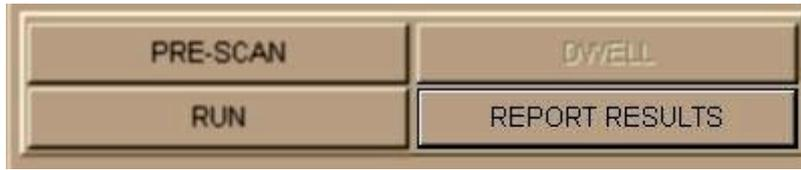
Once the scan is fully programmed, click on the REPORT RESULTS button to view the results of the test as the test proceeds. The target field strength profile will be displayed as a blue line.
