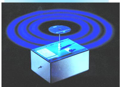
The ERS radiates a precisely known RF field strength and are supplied with calibration data measured at 3 metres. Their output is in the form of a closely spaced harmonic series which provides a series of continuous, narrowband signals covering the whole range.
