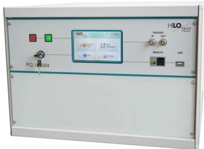
The Combination Wave Generator PG 12-804 is a combined impulse-current-/impulse-voltage generator which, for high-impedance loads,  $R_L > 100\Omega$ , delivers a standard impulse voltage with waveform 1.2/50 $\mu$ s and, for short-circuited output, a standard impulse current with waveform 8/20 $\mu$ s.
