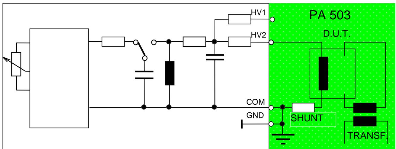
Fig. 2: Ring-Wave Generators IPG 612T, schematic, +Safety test cover PA 503, incl. modification of IPG 612T for testing RCCB's acc. to IEC 1008-1.
