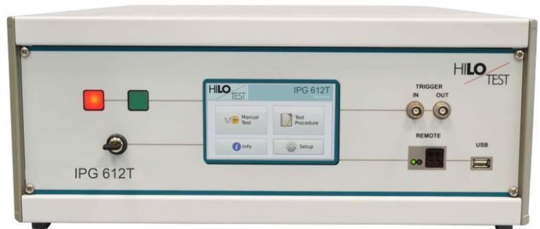
High-voltage pulse generator producing Ring Wave 0.5  $\mu$ s / 100 kHz acc. to IEC 61000-4-12. The output peak voltage can be preset continuously from 0.2 - 6 kV. Rise time 0.5 $\mu$ s to the first peak, ringing frequency 100 kHz.
