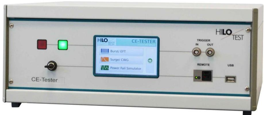
The Electrical Fast Transient Generator EFTG 4510 is a compact EMC test unit for testing electromagnetic immunity against electrical fast transients. The generator provides burst-pulses, which are adjustable in frequency, amplitude, duration and repetition rate. It is suitable to test the susceptibility levels of electrical systems and installations full compliant to IEC 61000-4-4.
