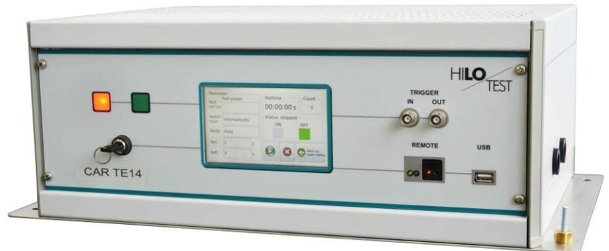
The CAR- Transient Emission 14 is used to check the transient transition behavior when switching loads on the vehicle electrical system. It consists of two triggerable circuit breakers (electronically or mechanically), an artificial network, a control unit for operating the device, and optionally an external power supply.
