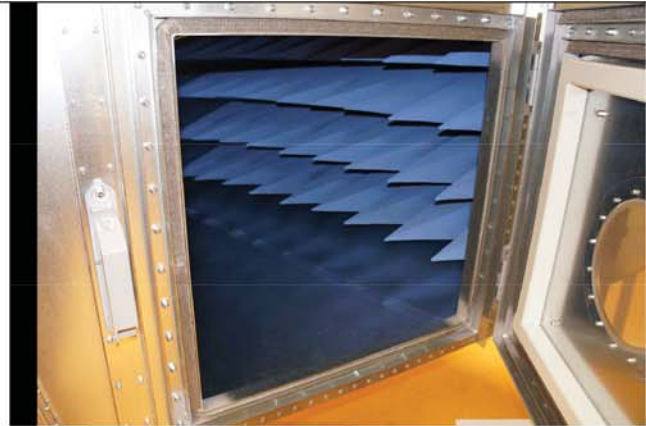
3 rows of gaskets with 3 mesh each
