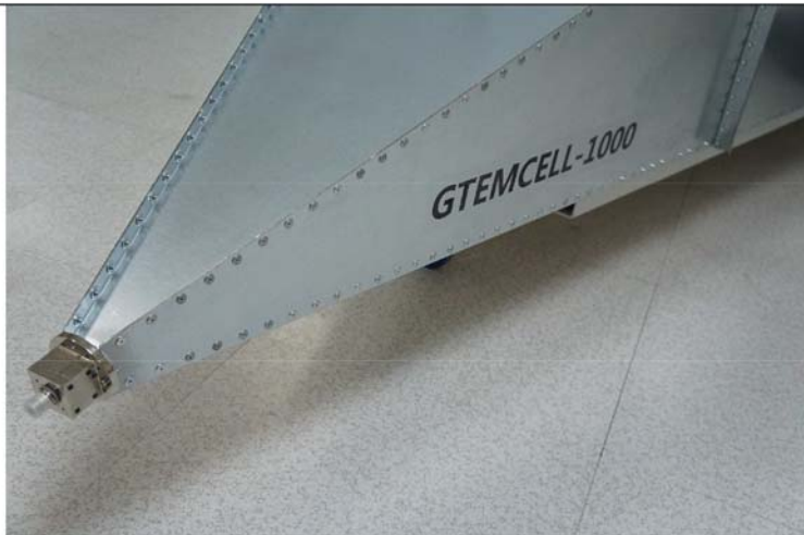
Special Multi-grip rivets system
