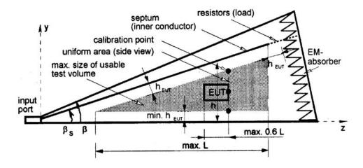
Fig.2 - Maximum EUT size and maximum size of the usable test volume in a GTEM cell, longitudinal section
