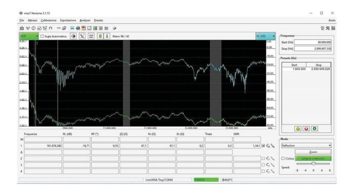
REFLECTION COEFFICIENT: S11 magnitude of GTEM-1750 in the range 80-3000MHz
