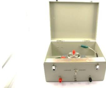
Fully shielded steel enclosure with high quality insulated surface for resistivity testing. This way the test can be done with little influence from the test environment.
