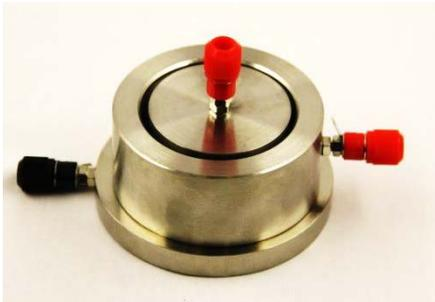
This concentric ring electrode is used for resistivity testing according to STM 11.11 and ANSI/ESD STM 11.12, ASTM D-257 and EIA-541.
