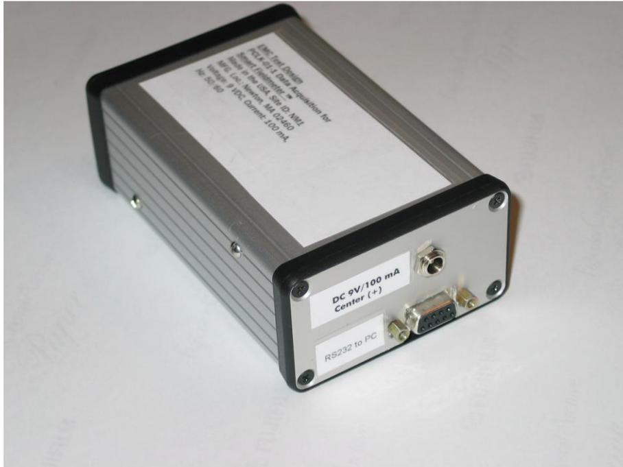
Introducing the Smart Fieldmeter [PC Link Kit: PCLK- 01-1 – low cost Option 1 solution](#) for simple connection of the Smart Fieldmeter to PC. This kit supports one Smart Fieldmeter unit and has into one stylish metal box containing the isolating differential amplifier (with more than 120 dB AC decoupling) and DAQ module acquiring 120 samples/sec with RS232 PC output. Software for data streaming, recording and archiving is included.
