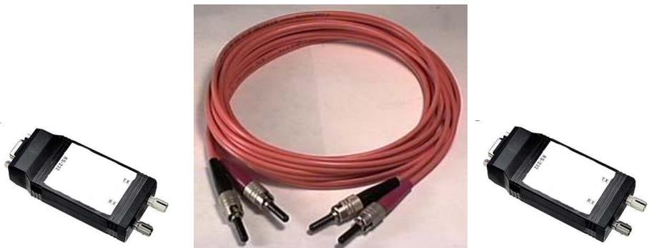
[Fiber Optic Link Kit: FOLK- 01 – the low cost Option 2 solution](#) to make fiber optic connection of Smart Fieldmeter to PC. Allows up to 100 ft. (30 meters) distance between screen room setup and equipment room PC. Kit includes two RS232/Optic converter units connected with bi-line fiber optic cable. Up-stream converter unit is connected to PC Link Kit PCLK- 01- 1, while down-stream unit is plugged directly into RS232 port of the PC.
