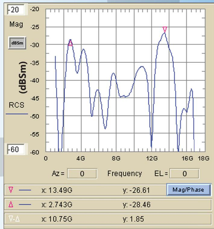
*Our amplitude frequency feature illustrates which frequencies the amplitude of your RCS profile are highest and lowest from measurement data.*
