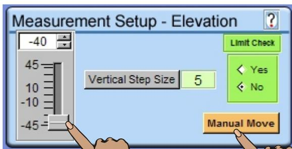
Position the platform to -40 deg using the slider or the constant and "Manual Move"
