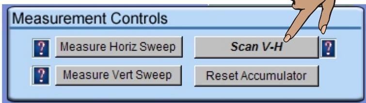
Invoke the Scan function. The scan V-H button will stay depressed until the measurements are complete.
