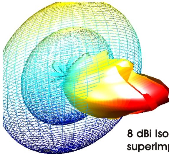
8 dBi Isosphere superimposed over linear  $S_{21}^2$  patch antenna
