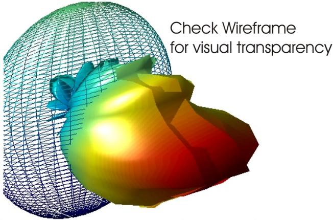
6 dBi Isosphere superimposed over linear  $S_{21}^2$  patch antenna
