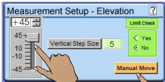
Set the Elevation slider to +40 deg. but do not move the platform. The platform will step to +45 deg during the Scan. Note that TOP SCAN stop = +45 deg is past the top of the top of the antenna. It is only necessary to end at 0 deg.
