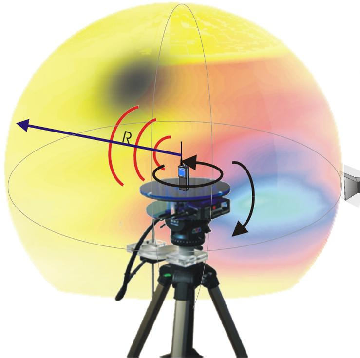
The Map To Sphere feature projects the  $S_{21}^2$  response on to the unit sphere. This is useful for determining the beam width for any level relative to the maximum.
