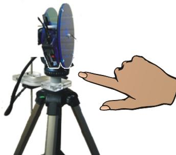
Tilt the double jointed tripod to -90 degrees and reposition the tripod so that the original antenna under test phase center is maintained
