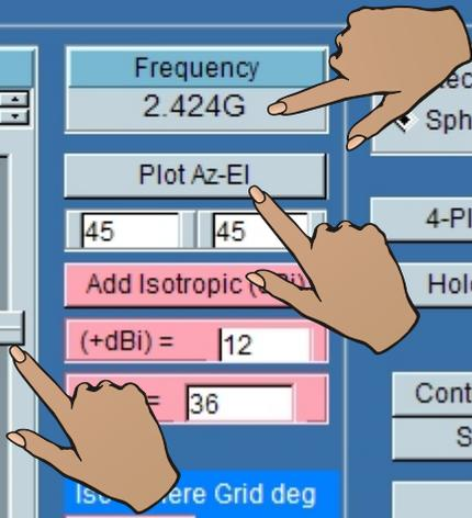
The AZ-EL plotting menu will appear. Slide the frequency slider to the desired frequency and invoke Plot Az-EL
