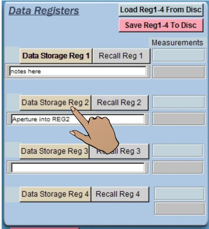
Save the scan data to REG2. Note that it is necessary to have the side scan in REG1 and the Top scan in REG2.
