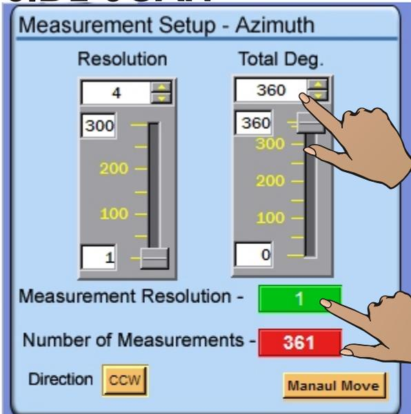
Set the Az rotation to 360 deg and the resolution to 1 degree. The DAMs will make a frequency sweep every 1 degree.
