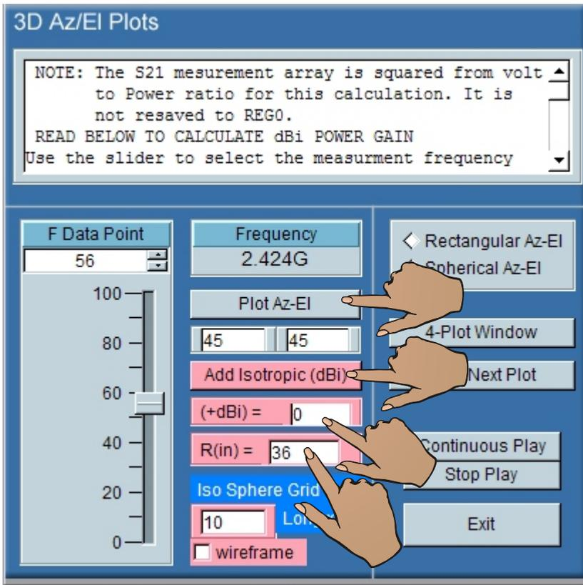
Generate an isotropic sphere by entering the antenna separation and the sphere gain 0 dBi. Depress Add Isotropic (dBi) and re-plot previous
