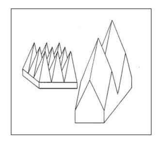
square 24 inch (610 mm) panels. SFC-48 is available as a standard pyramid or in the twisted pyramid design with an 18x36 inch (457 x 914 mm) base dimension. Larger sizes are a "twisted pyramid" design which improves the wide angle performance and, because of the extended shoulder height, exhibits less drooping of the tips after installation.
