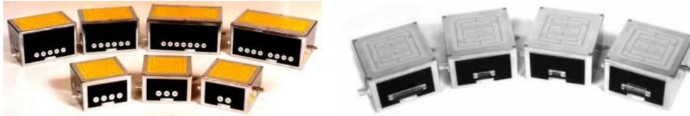
Designed specifically to meet the conducted RF immunity testing conditions specified in EN61000-4-6: 1996. These units are able to handle 20V rms up to 80 MHz, 10V upto150 MHz and 3V rms up to 230 MHz. Options include internal 6 dB 50 ohm RF power pad. Supplied with a certificate of conformity, calibration results, level setting data and connectors.
