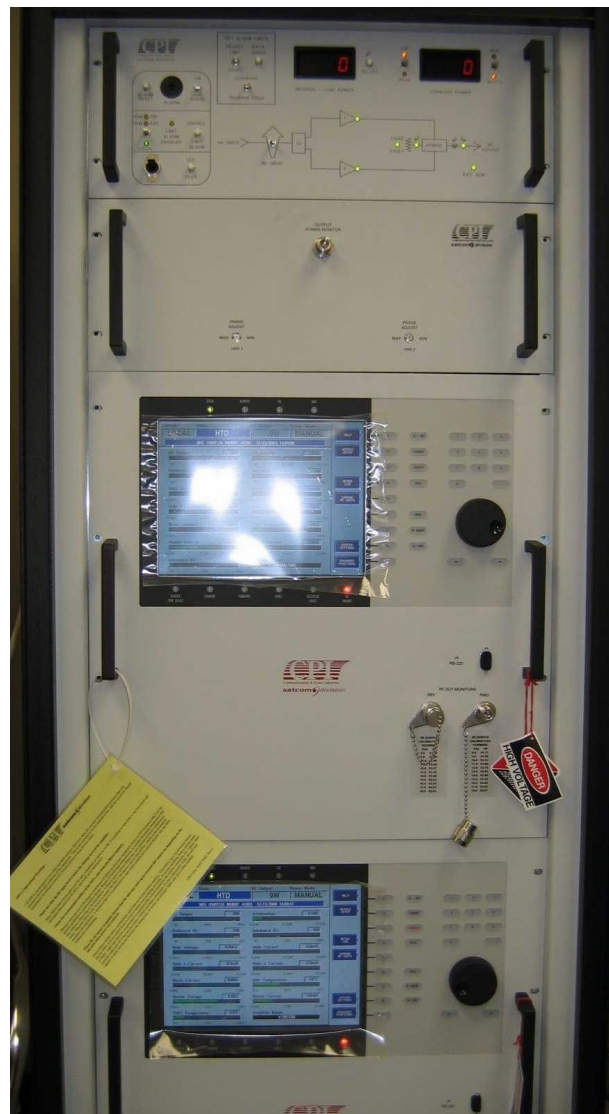
CPI 900 W L-band TWTA System, Model VZL2780P2
