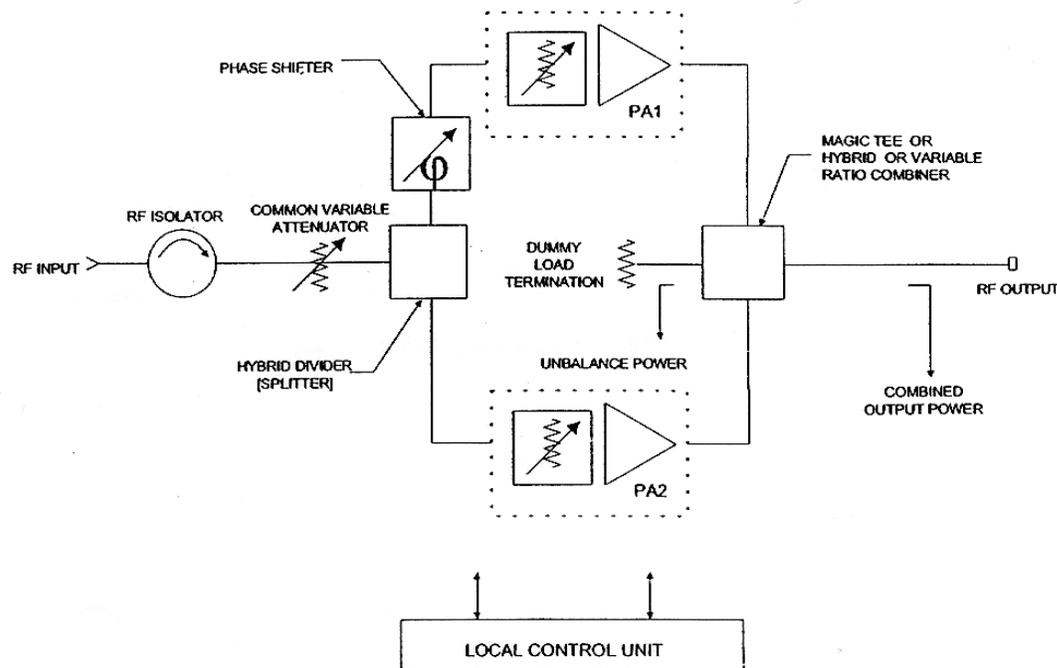
*Figure 1. Block Diagram, Basic Power Combiner Circuit*
