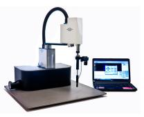
**SmartScan Basic** is a manual system with manual data record capability. The user can take the DUT picture and probe position pictures to add comments to each failing location.
